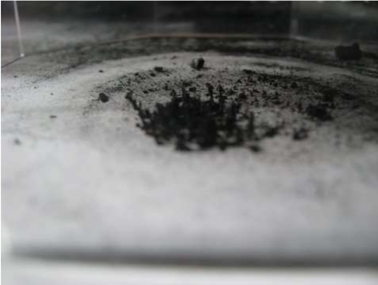
A side view through the container, shows the carbon trees standing.
