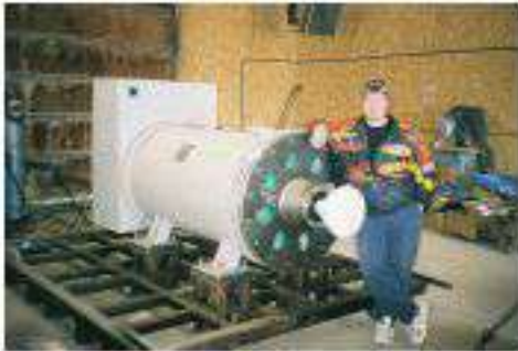
This is the size of the 1.2 MWe alternator compared to one of the team
