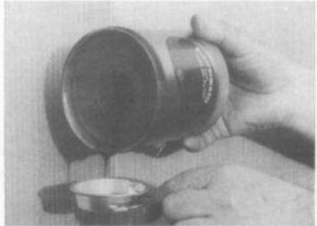
Taking the oil sample for the CRACKLE TEST
