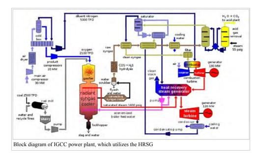
The gasification process can produce syngas from a wide variety of carbon-containing feedstocks, such as high-sulfur coal, heavy petroleum residues and biomass.
