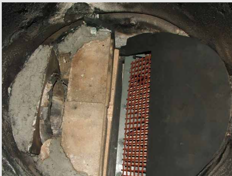
This is a trial assembly. It was re-done. It does show how the first s.s. screen sits in the slot of the screen support plate. Notice that the lower edge of the screen is behind the 'fingers' of the grate shaker plate.
