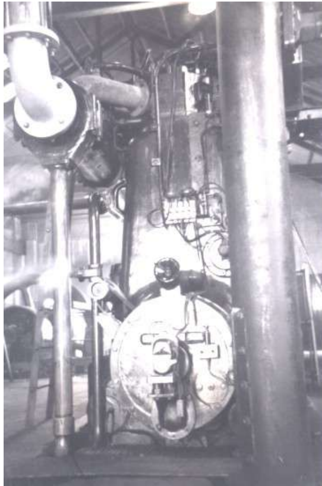
Photo 7. No.1 National Engine Dual ignition system visible Note a vague picture of Crossley No. 3 rear left
