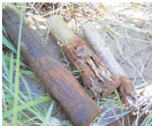
Figure 3: Preservative tests using slow pyrolysis liquid that have been running for more than two years (left pole treated with pyrolytic material from RWC's plant)
