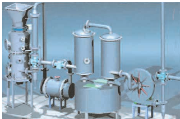
Figure 3: Pilot scale downdraft biomass gasifier
