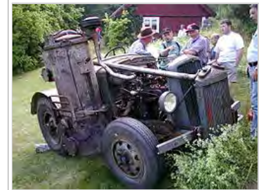
Wood gasifier on a Ford truck converted into a tractor
