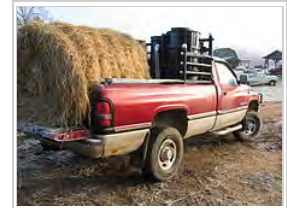
Dodge V10 hauling hay with woodgas. Keith gasifier system.
