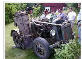
Imbert gasifier on a Ford truck converted to a tractor
