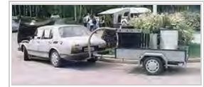
Saab 99 running on wood gas in Finland. The gas generator is on the trailer.
