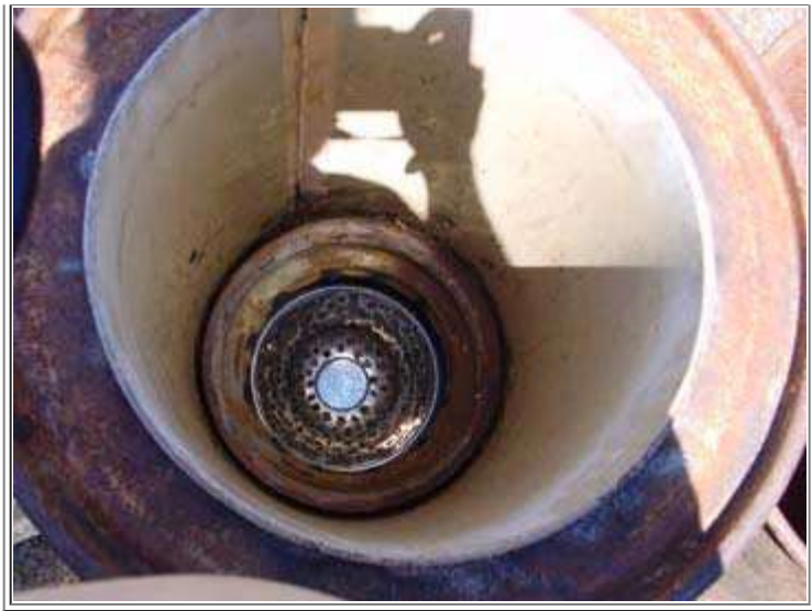
a view down into the gassifier core
