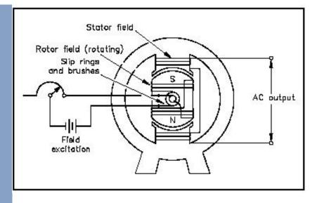
Figure 3 Simple AC Generator
