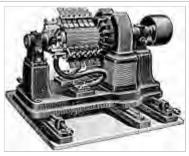
This large belt-driven highcurrent dynamo produced 310 amperes at 7 volts. Dynamos are no longer used due to the size and complexity of the commutator needed for high power applications.
