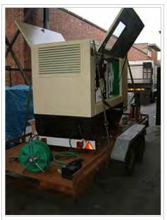
Side view of a large Perkins diesel generator, manufactured by FG Wilson Engineering Ltd. This is a 100 kVA set
