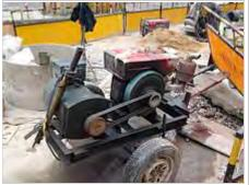
Cart-mounted enginegenerator being used at a construction site very large units may start with compressed air either to an air driven starter motor or introduced directly to the engine cylinders to initiate engine rotation. Standby power generating units often include an automatic starting system and a transfer switch to disconnect the load from the utility power source when there is a power failure and connect it to the generator.
