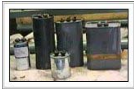
Typical Running Capacitors...GOOD! .....Starting cap...Bad!
