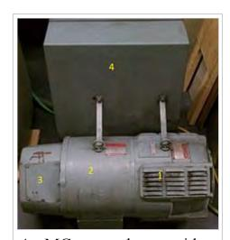
An MG set used to provide a variable three phase AC voltage for an Electron Beam Welding Machine high voltage power supply.
