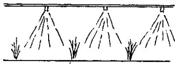
Figure No. 29 Height and the State for spraying 1) good condition
