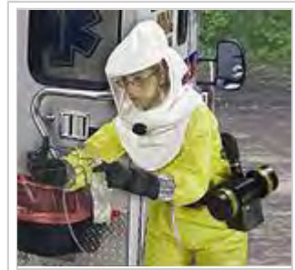
PAPR with hood. APF decreased from 1000 to 25 after PF studies in the workplaces
