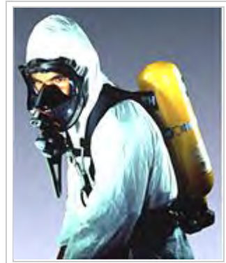
Self Containing Breathing Apparatus (SCBA) with pressure-demand air supply mode into the full face mask. This is the most reliable RPD type, its APF = 10 000
