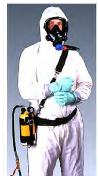
Supplied Air Respirator (SAR) with auxiliary breathing apparatus (for evacuation in case of possible supply disruptions of air through the hose) with pressure-demand air supply mode into the full face mask. This is one of the most reliable RPD type, its APF = 1000
