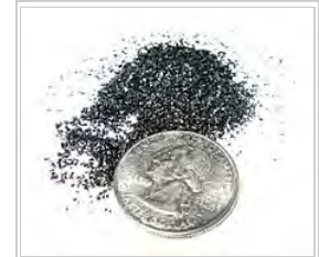
Black powder for muzzleloading rifles and pistols in FFFG granulation size. U.S. Quarter (diameter 24 mm) for comparison.
