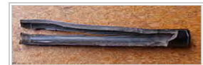
Burst barrel of a muzzle loader pistol replica, which was loaded with nitrocellulose powder instead of black powder and could not withstand the higher pressures of the modern propellant
