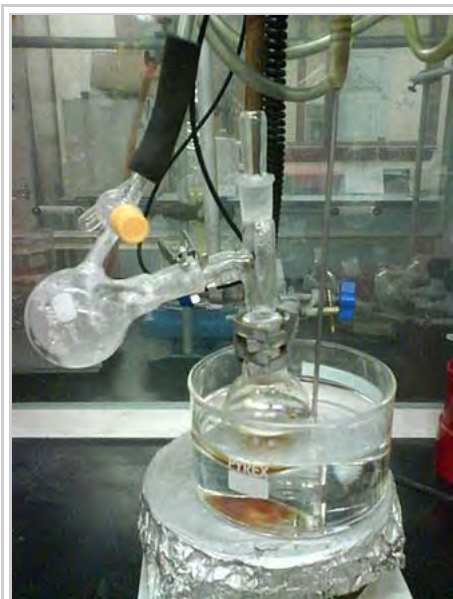
Dimethyl sulfoxide usually boils at 189 °C. Under a vacuum, it distills off into the receiver at only 70 °C.
