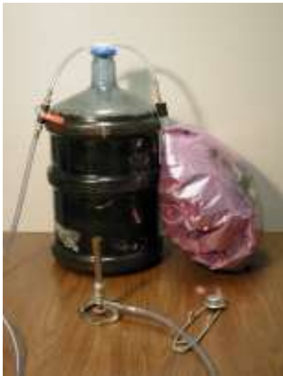
Completed biogas generator.
