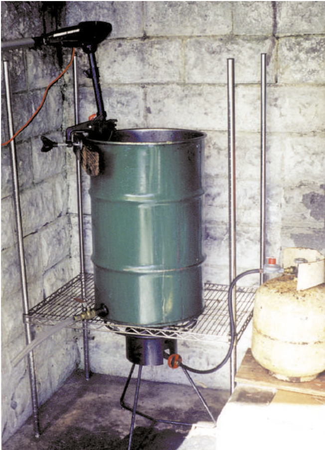
In the reactor tank, ingredients are mixed with an electric outboard motor and heated with a propane burner.
