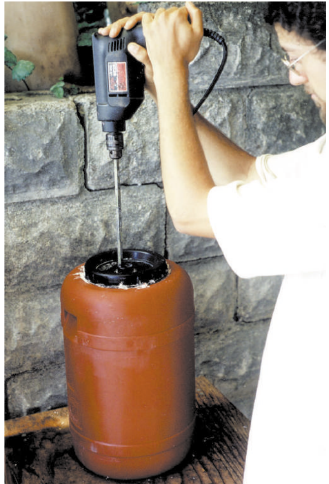
Panama uses a paint mixer to combine methanol and lye in a closed container to make sodium methoxide. In this posed photo, he skipped the usual protective gear.
