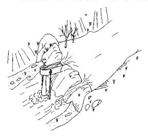
Dams have both advantages and disadvantages. If used in a village setting they can provide additional uses as a fish pond and washing area. The dam wall may support a row of PowerPal generators so that several families can have access to electricity. If the village works together to build the dam the time and construction costs are lower. Dams are less likely to be effected by flooding if diversion channels are adequate, so PowerPal can be used effectively during the rainy season.
