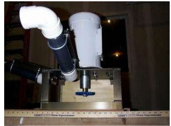
Nozzles retracted to show runner, arbor and coupling arrangement for connection to motor shaft.
