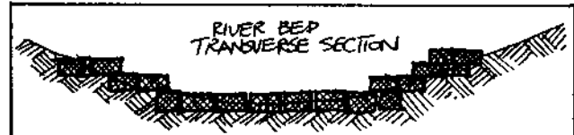
FIGURE 7.13 CHECK DAM FOR RAM PUMP OR WATER WHEEL Only 1–3 m of head enables modest energy use for mechanical power, lift pumps, or diversion to canals.
