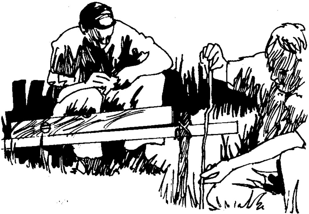
A simple method of measuring head. With a straightedge held level, the vertical height between a pair of pegs is read off and noted.
