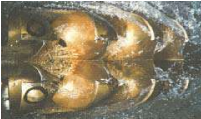
Fig. 3: A stroboscopic photograph of water distribution in a Pelton wheel, showing water sheets leaving buckets.
