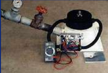
Stream Engine showing multi-meter (included) used to measure output current.
