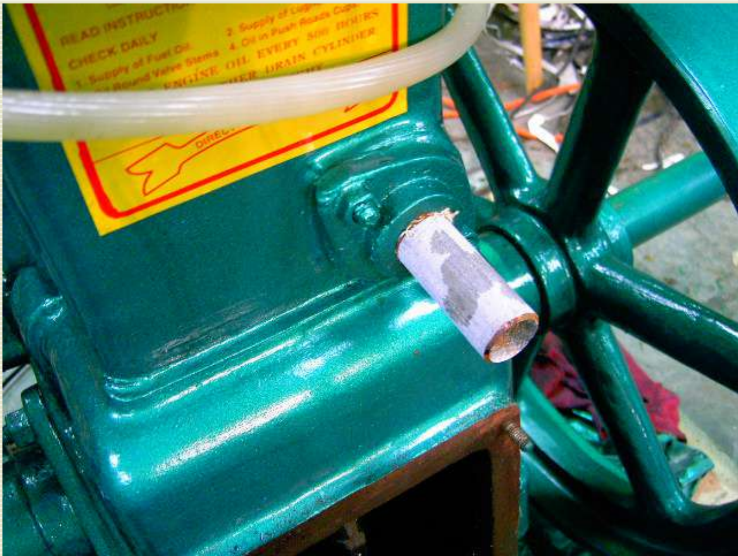
Shot of lower coolant inlet. I removed this lower coolant fitting and looked inside the cylinder, very well made casting.
