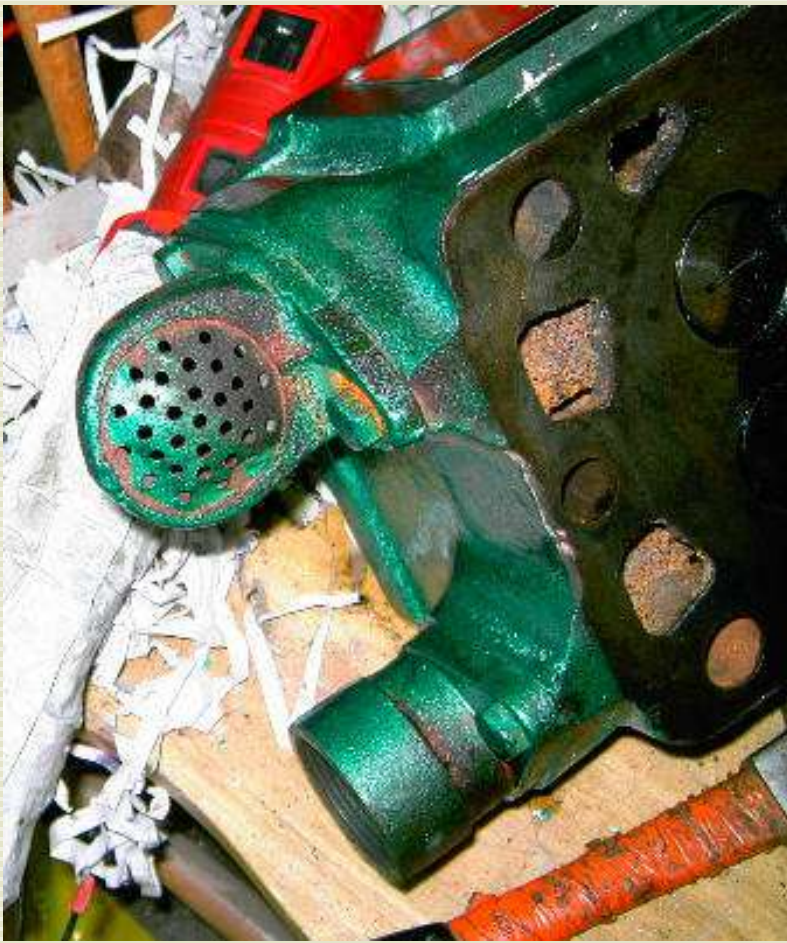
Above: Is the air inlet, standard bolt pattern and flange, you should plan to add your own filter, easy to do.
