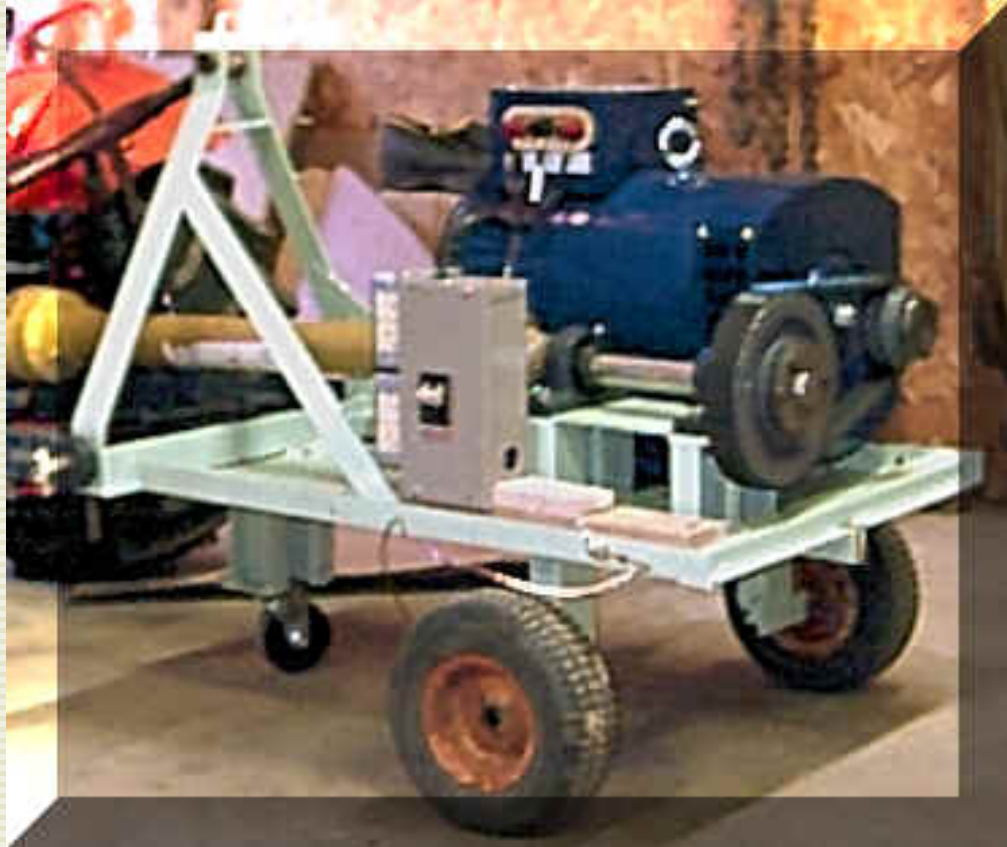
Mark has mounted and wired in a breaker box, It looks like he has also attached some metal boxes to the side of the breaker box to house some plug ins, also note his ground wire.
