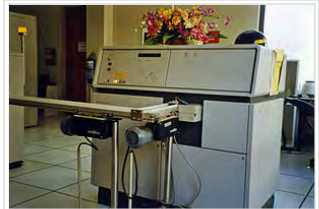
Online X-ray diffraction with automatic sample feed for free calcium oxide measurement
