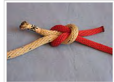
The reef knot can capsize if one of its standing ends is pulled.
