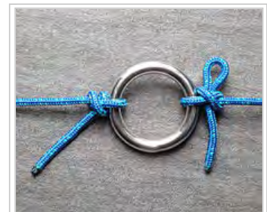
The slipped form of the buntline hitch (on the right) can easily be untied by pulling the hanging end and withdrawing the loop.
