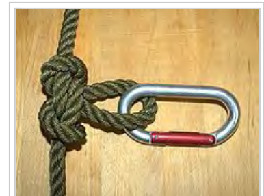
The alpine butterfly loop is a knot that can be tied on the bight.
