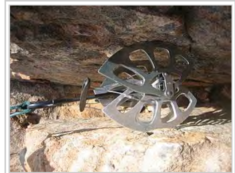
An SLCD placed in a crack.
