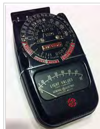
General Electric Light Meter used in photography to measure light values in foot candles.
