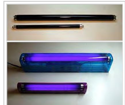
Two black light fluorescent tubes, showing use. The top is a F15T8/BLB 18 inch, 15 watt tube, used in a standard plug-in fluorescent fixture. The bottom is an F8T5/BLB 12 inch, 8 watt tube, used in a portable battery-powered black light sold as a pet urine detector.
