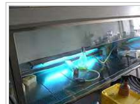
A low-pressure mercury-vapor discharge tube floods the inside of a biosafety cabinet with shortwave UV light when not in use, sterilizing microbiological contaminants from irradiated surfaces.
