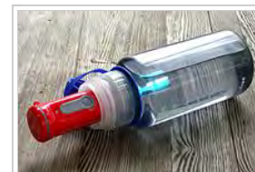
A portable, battery-powered, low-pressure mercury-vapor discharge lamp for water sterilization.
