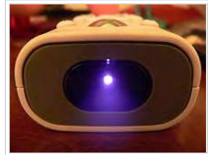
Infrared light from the LED of a remote control as recorded by a digital camera.
