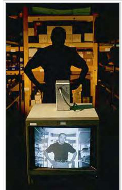
Active-infrared night vision : the camera illuminates the scene at infrared wavelengths invisible to the human eye. Despite a dark back-lit scene, active-infrared night vision delivers identifying details, as seen on the display monitor.
