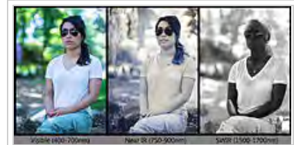
Reflected light photograph in various infrared spectra to illustrate the appearance as the wavelength of light changes.
