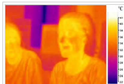
A false color image of two people taken in long-wavelength infrared (body-temperature thermal) light.
