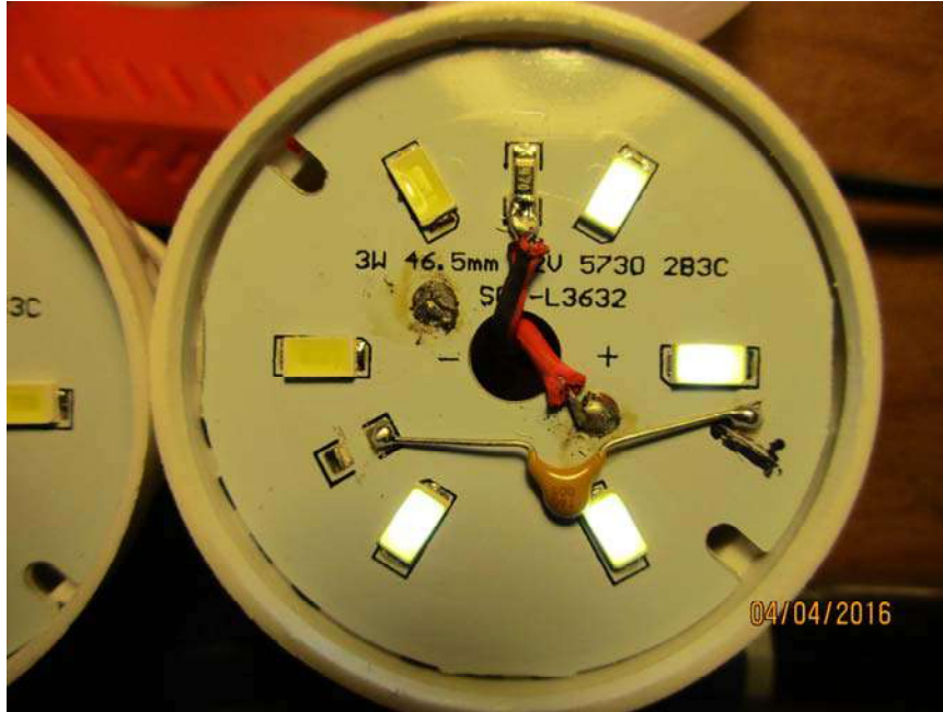
This is a close up of the round configuration after being modified.
