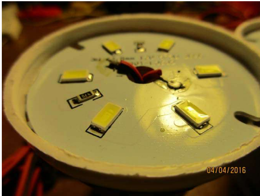
This shows how one can tip the unit it an angle to get a reflection of light to show where the copper printed circuit path is.
