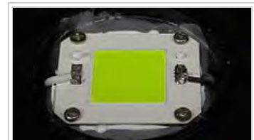
An 80W Chip-On-Board COB LED Module from an industrial light luminaire, thermally bonded to the heat sink.
