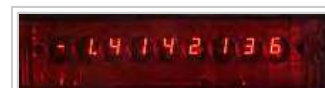
LED display of a TI-30 scientific calculator (ca. 1978), which uses plastic lenses to increase the visible digit size
