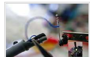
Green electroluminescence from a point contact on a crystal of SiC recreates Round's original experiment from 1907.
