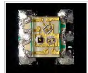
Very small (1.6x1.6x0.35 mm) red, green, and blue surface mount miniature LED package with gold wire bonding details.
