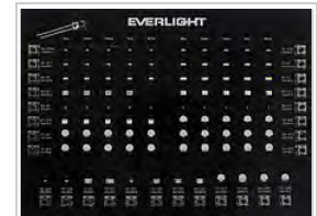
Photo of miniature surface mount LEDs in most common sizes. They can be much smaller than a traditional 5 mm lamp type LED which is shown on the upper left corner.
