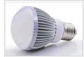
A bulb-shaped modern retrofit LED lamp with aluminium heat sink, a light diffusing dome and E27 screw base, using a built-in power supply working on mains voltage
