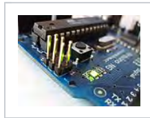
A green surface-mount colored LED mounted on an Arduino circuit board
