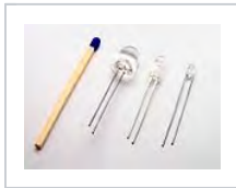
Different sized LEDs. 8 mm, 5 mm and 3 mm, with a wooden match-stick for scale.
