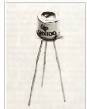
A Texas Instruments SNX-100 GaAs LED contained in a TO-18 transistor metal case.
