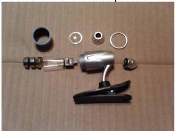
Keep the clip, case, plastic lens, reflector cone and screw on front ring. Toss aside the rest. You might be able to use the switch on another project.
