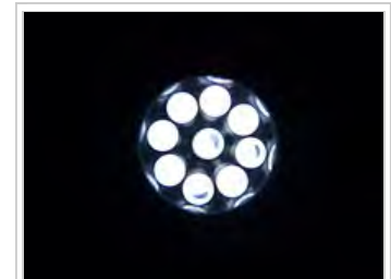
Multiple 5 mm LEDs may be used in small flashlights.
