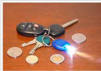
Miniature LED flashlight on a key chain, powered by lithium primary coin batteries.
