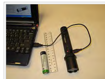
An LED flashlight which can charge and also have certain functions programmed via the USB port. The user can select stages of brightness level or flashing frequency through vendor supplied software running on a computer. A spare 18650 size lithium-ion rechargeable battery is also shown.
