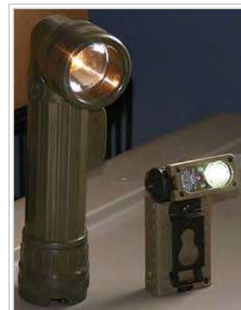
The angle-head flashlight on the left uses an incandescent bulb, while the adjustable angle-head flashlight on the right uses LEDs to give white, red, blue, and infrared light
