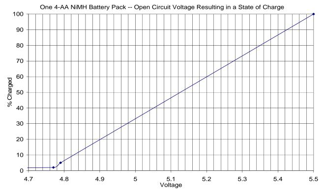
A simplistic way of charging is to use a resistor in series to limit current. If this is done the following is a typical result.
