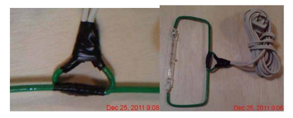
Use number 10 gauge solid copper single stranded insolated copper wire. Bend it as show above. When the two pieces are soldered to an extension cord and taped as shown they become stiff enough to be able to hold a 150, 300 or 500 watt tungsten light bulb.
