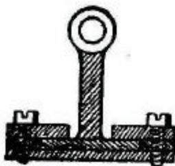
FIG. 64. — Cross section of crosshead and guide.
