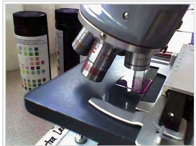
A typical histologic specimen, mounted between a glass microscope slide and a glass coverslip, positioned on the stage of a light microscope.
