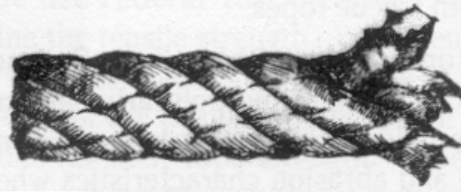
Three strand twisted or laid rope.
