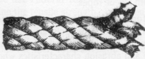
Three strand twisted or laid rope.
