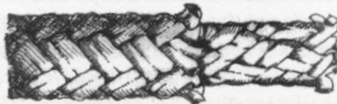
Double braid rope showing the braided sheath and braided core.
