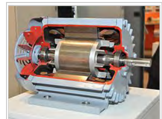
Cutaway view through stator of TEFC induction motor. Note rotor air circulation vanes. Many such motors have a symmetric armature, and the frame may be reversed to place the electrical connection box (not shown) on the opposite side.
