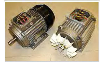
Three-phase totally enclosed fan-cooled (TEFC) induction motor with end cover on the left, and without end cover to show cooling fan. In TEFC motors, interior losses are dissipated indirectly through enclosure fins mostly by forced air convection.
