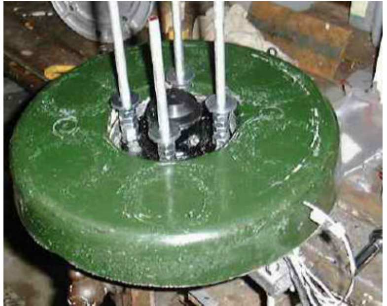
Fitting the stator
