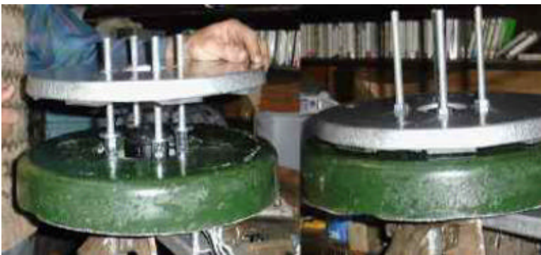
Fitting the front magnet rotor
