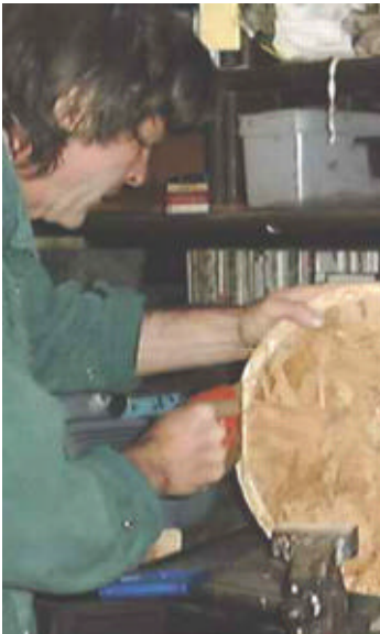
Sawing flat faces on the inner mould
