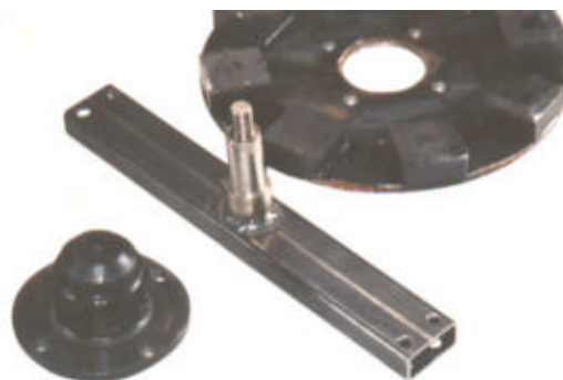
Spine, shaft, hub and magnet rotor
