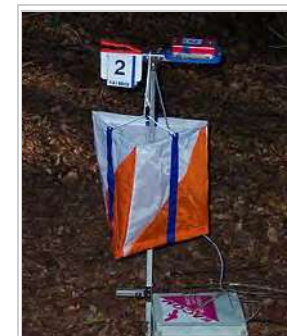
A transmitter, orienteering control flag, paper punch and electronic punch device at an ARDF control.
