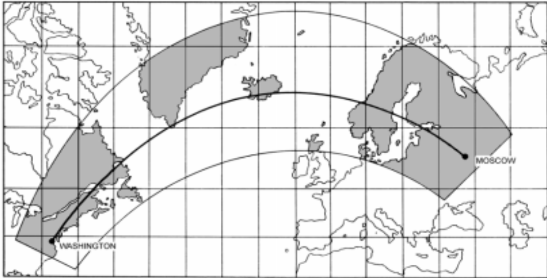
Figure 309c. The great circle between Washington and Moscow as it appears on a Mercator map.
