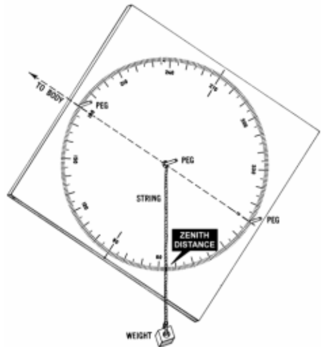
Figure 2608b. Improvised astrolabe; direct sighting method.
