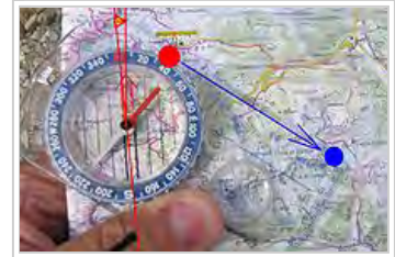
Turning the compass scale on the map (D – the local magnetic declination)
