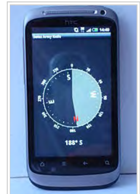
A smartphone that can be used as a compass because of the magnetometer inside.
