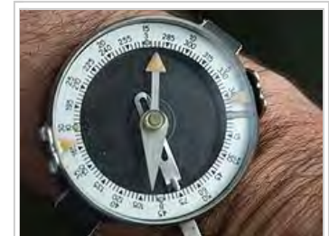
Wrist compass of the Soviet Army with counterclockwise double graduation: 60° (like a watch) and 360°
