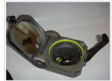
A standard Brunton Geo, used commonly by geologists
