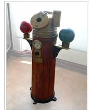
A binnacle containing a ship's standard compass, with the two iron balls which correct the effects of ferromagnetic materials. This unit is on display in a museum.
