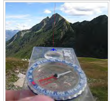
When the needle is aligned with and superimposed over the outlined orienting arrow on the bottom of the capsule, the degree figure on the compass ring at the direction-of-travel (DOT) indicator gives the magnetic bearing to the target (mountain).
