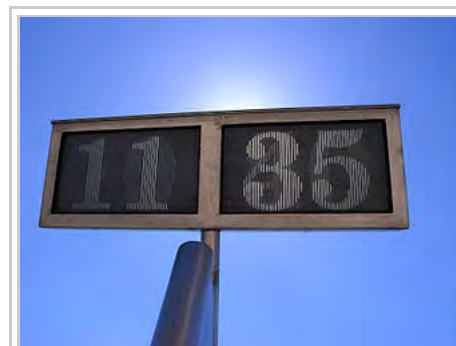
This sundial by Digital sundials international uses just two masks and a plexiglas layer.
