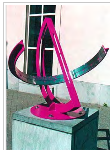
Equatorial bow sundial in Hasselt, Flanders in Belgium 50°55′47″N 5°20′31″E. The rays pass through the narrow slot, forming a uniformly rotating sheet of light that falls on the circular bow. The hour-lines are equally spaced; in this image, the local solar time is roughly 15:00 hours (3 pm). On September 10, a small ball, welded into the slot casts a shadow on centre of the hour band.
