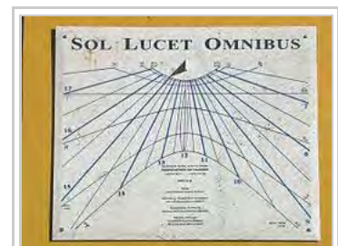
Vertical reclining dial in the Southern Hemisphere, facing due north, with hyperbolic declination lines and hour lines. Ordinary vertical sundial at this latitude (between tropics) could not produce a declination line for the summer solstice.
