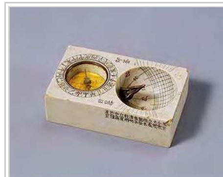
Angbuilgu , a portable sundial used in Korea during the Joseon period. The integrated magnetic compass aligns the instrument toward north pole.(National Museum of Korea) [88]
