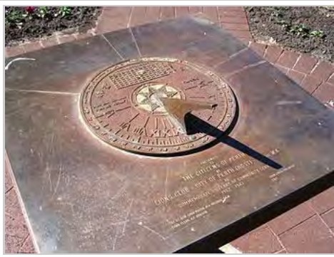
Southern-hemisphere sundial in Perth, Australia. Magnify to see that the hour marks run anticlockwise. Note graph of Equation of Time, needed to correct sundial readings.
