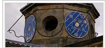
Two vertical dials at Houghton Hall Norfolk UK 52°49'39"N 0°39'27"E. The left and right dials face South and East, respectively. Both styles are parallel, their angle to the horizontal equaling the latitude. The East-facing dial is a polar dial with parallel hour-lines, the dial-face being parallel to the style.
