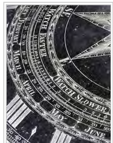
The Whitehurst & Son sundial made in 1812, with a circular scale showing the equation of time correction. This is now on display in the Derby Museum.
