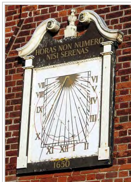
SSW facing, vertical declining sundial on Moot Hall, Aldeburgh, Suffolk, England. The gnomon is a rod that is very narrow, so it functions as the style.
