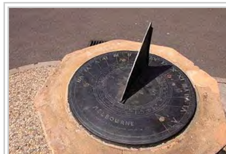
In this sundial, in Melbourne, Australia, the gnomon is the triangular blade. The style is its inclined edge.
